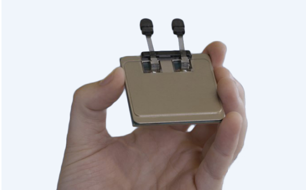
Figure 2 - Example Multi-Chip Package Assembly with TeraPHY™ Optical I/O
